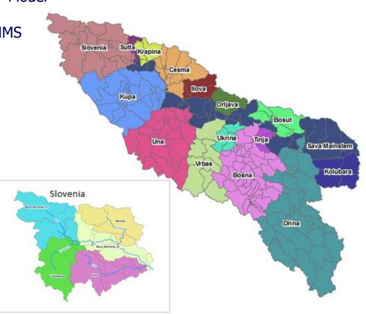
Final HEC-HMS Model contains a separate basin models for each tributary basin and mainstem reach (22 models in total)
